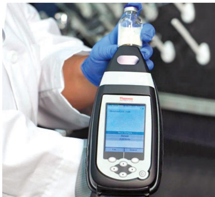
Thermo Scientific's microPHAZIR RX can provide raw material identification in seconds
