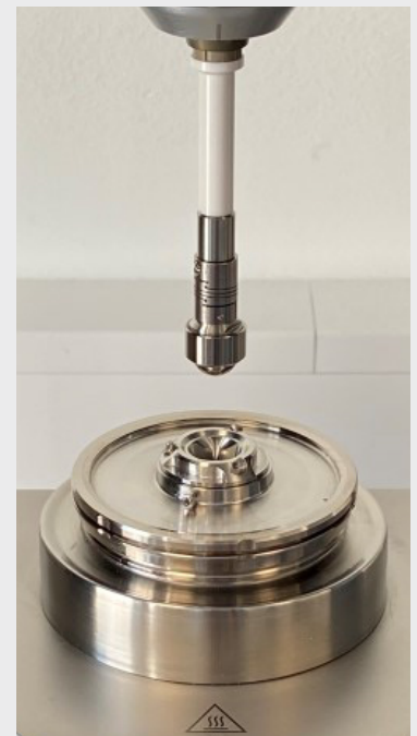
Figure 3: Tribology measuring geometry consisting of a ball on three plates setup.
