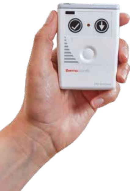
**Electronical dosimeters EPD Trudose G and EPD Trudose BG have the capability to warn the user if he is exposed to an instrument overrange condition in direct beam and accumulate the dose correctly outside the direct beam area.**
