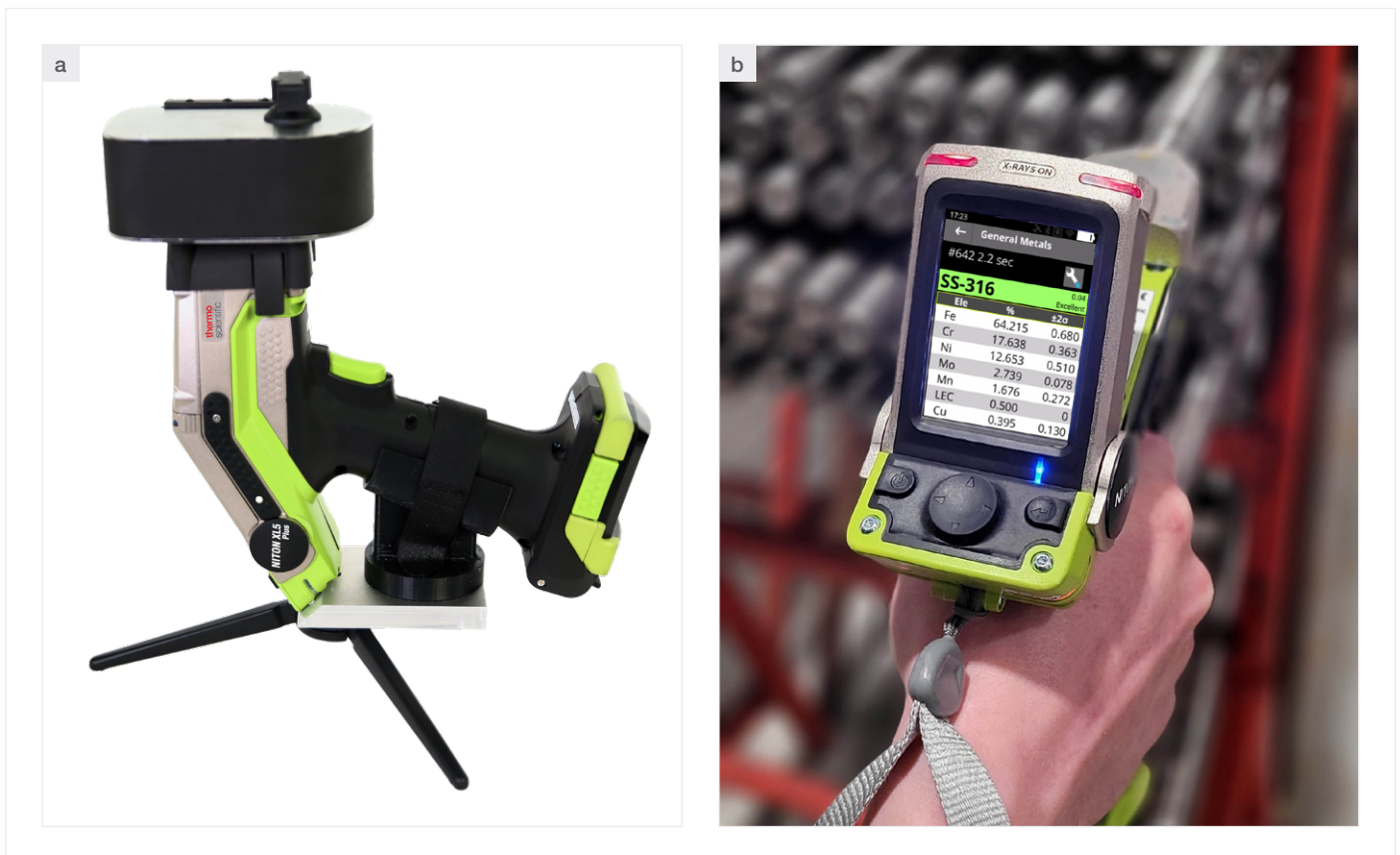
Figure 4. (a) The Niton XL5 Plus Handheld XRF Analyzer with a sample loaded in test stand; (b) Live readout of stainless steel 316 and its elemental composition on the Niton XL5 Plus Analyzer.
