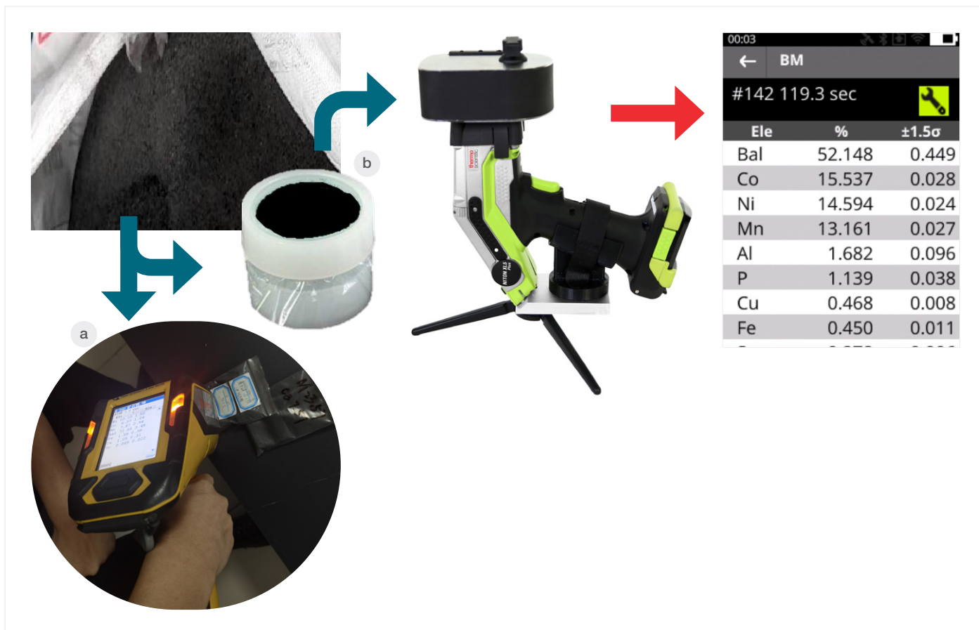
Figure 2. Workflow for rapid analysis of black mass: (a) semi-quantitative analysis of black mass in bags (base metals such as copper, nickel, cobalt, or manganese) using the Niton XL2 XRF Analyzer; (b) quantitative analysis of the full element range from Mg-U in sample cups using the Niton XL5 Plus XRF Analyzer.
