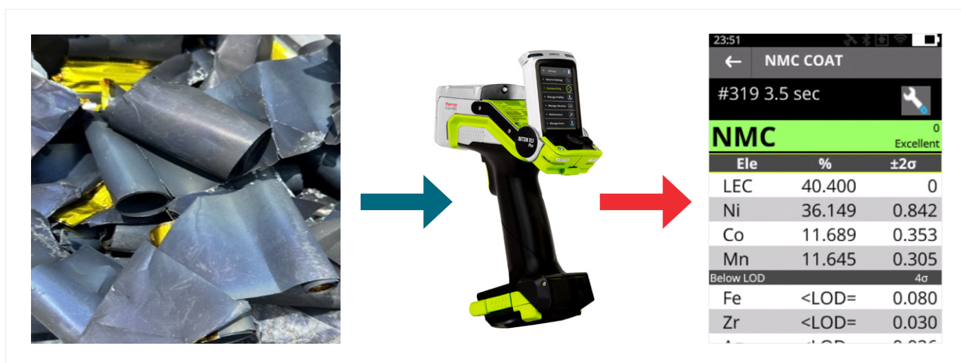
Figure 1. Sorting production scrap with HHXRF by identifying types of scrap cathode films.
