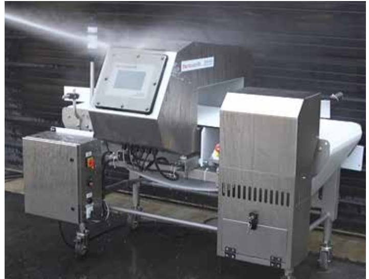
Example of high pressure washdown.
