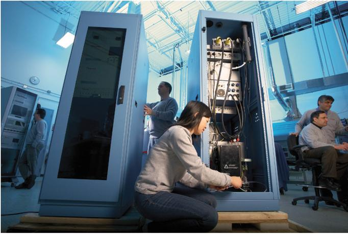
File image showing the manufacturing of a Thermo Scientific mercury CEMS system.
