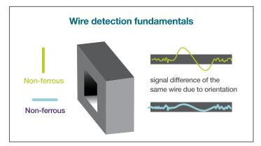
During production, contaminants can come in many shapes and sizes and composed of different metal materials. There are endless possibilities of foreign objects, making it impossible to predict how metal contamination will manifest. Thus, production facilities must respect the unpredictable nature of orientation effect and consider their inspection system's ability to address this concern.
