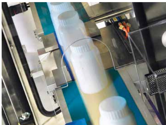
Plastic tablet bottles being weighed on an inline checkweighing system.
