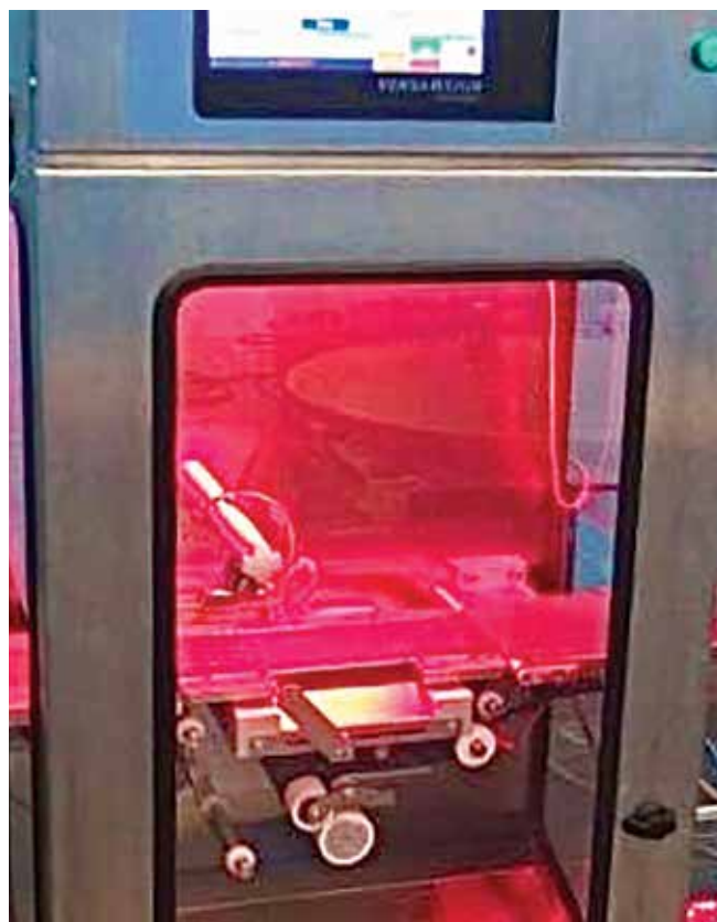
Colored, internal lighting provides an easily visible indication of the operating status of a checkweigher system.
