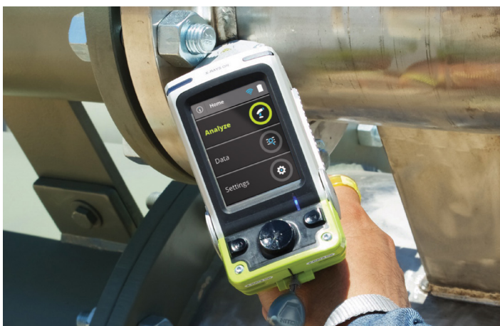
The Thermo Scientific™ Niton™ XL5 handheld XRF analyzer in use validating incoming materials to ensure material specifications are met.
