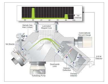
Figure 1 Prima PRO's magnetic sector analyzer
