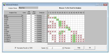
Figure 4 Example of flare stream method
