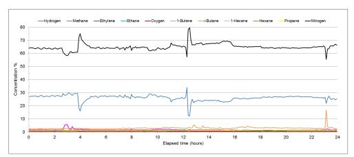
Figure 7 24-hour trend display of flare gas stream
