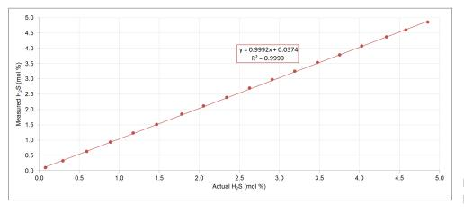
Figure 9 Linearity plot for H<sub>2</sub>S from 800 ppm to 4.85%
