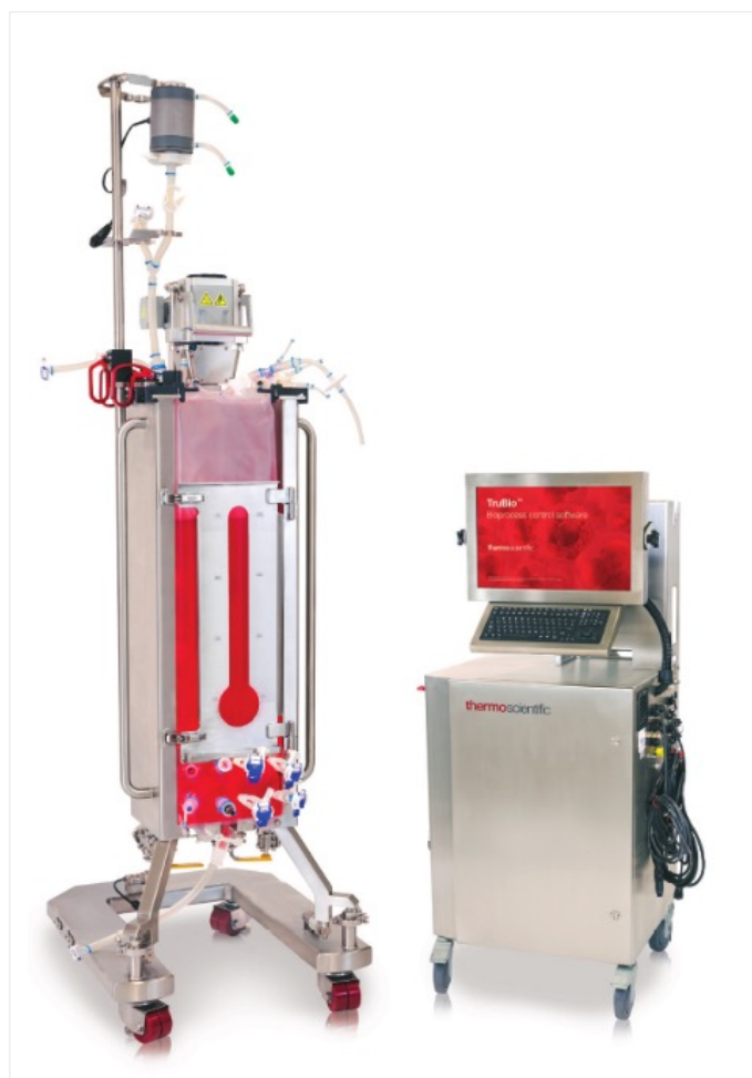
Figure 2. 50L Thermo Scientific DynaDrive S.U.B. for cell culture applications.
