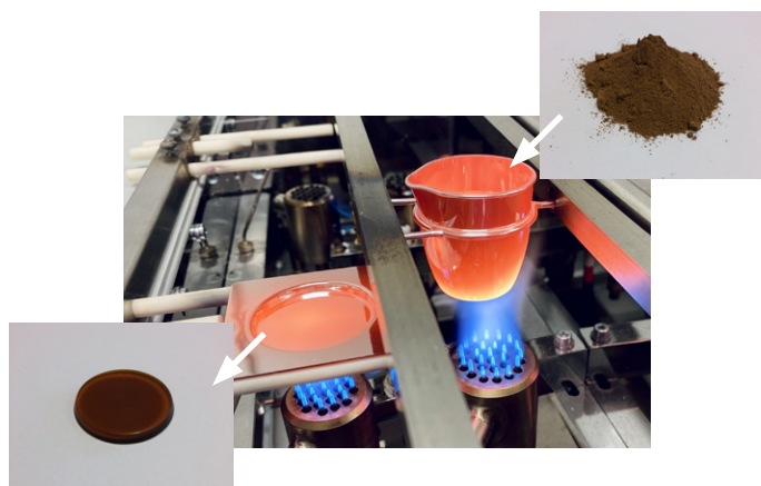
Figure 2. Transformation of the powder material into a glassy sample by fusion at high temperature.
