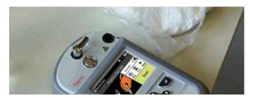
A quick TruNarc scan produces a 'fingerprint' of the substance being evaluated at the time. Gemini has a proprietary database that allows great precision in the verification of chemical substances. When used in combination, for example, one can determine immediately if a seized pill is part of the pharmaceutical legal industry or if it is an illegal drug.
