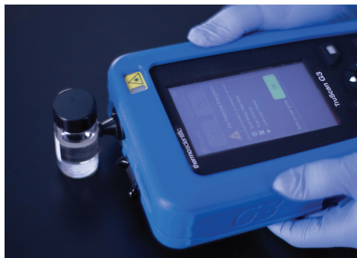
Raman analysis is non-contact through polybags, plastic or glass and can measure liquids, emulsions, gels and solids in seconds.
