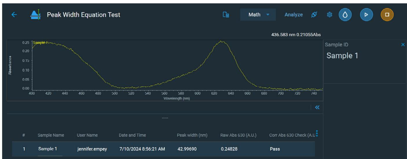
Figure 2. Measurement window displaying the peak width calculation, the raw absorbance at 630 nm, and a Pass/Fail test. The data reported here is simulated to demonstrate the software capabilities.
