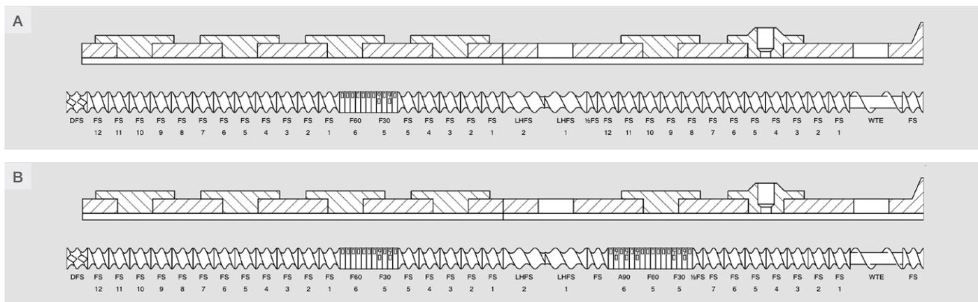
**Figure 5. Schematic diagram of the screw configurations used in the TSG.**
