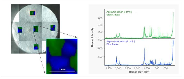
Figure 10. FT-Raman mapping of 5 regions on a commercially available migraine tablet. The MCR images show the distribution of the two largest components (acetaminophen – Form I (green) and aspirin (blue)).
