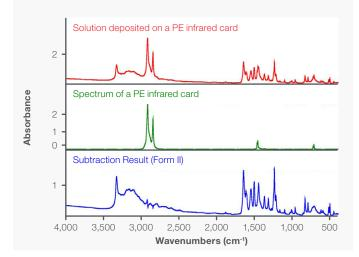
Figure 3. Mid-IR transmission spectra for a methanol solution of acetaminophen deposited on a PE IR card, a blank PE card, and the subtraction result (Form II).
