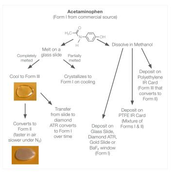
Figure 1. Routes to produce different polymorphic forms of acetaminophen.
