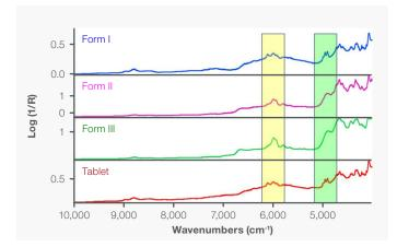
Figure 8. NIR diffuse reflection spectra of Forms I, II, and III of acetaminophen and a commercial acetaminophen tablet.
