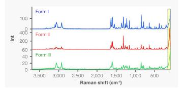
Figure 9. FT-Raman spectra of Forms I, II, and III of acetaminophen.
