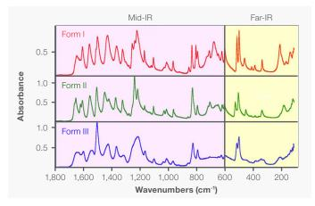
Figure 6. Far-IR diamond ATR spectra of the three polymorphic forms of acetaminophen.
