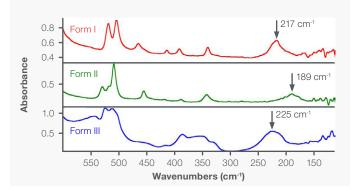
Figure 5. Far-IR transmission spectra of Forms I, II, and III of acetaminophen on PE IR cards.
