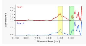
Figure 7. NIR transmission spectra of Forms I and II of acetaminophen on glass slides.
