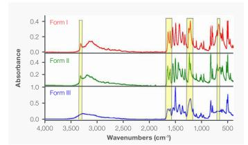
Figure 2. Mid-IR diamond ATR spectra of Forms I, II, and III. The regions highlighted in yellow show the difference between the spectra.
