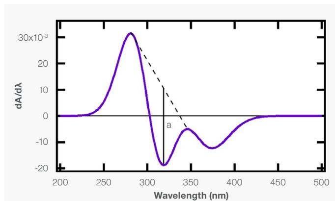
Figure 8. Tangent Method Diagram.
