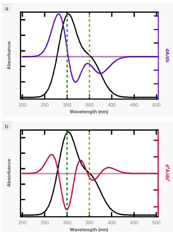
**Figure 2. Calculated UV-Visible absorption spectrum (black line) compared to the (a) first and (b) second derivative of the calculated spectrum. Dashed green and orange lines correspond to the location of the maxima for component A and component B, respectively. The dashed horizontal line indicates where the first and second derivatives equal 0.**
