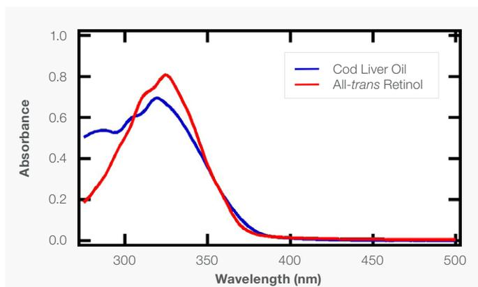
Figure 5. UV-Visible absorption spectrum of retinol (red) and cod liver oil (blue) measured in a 1.0 cm quartz cuvette.
