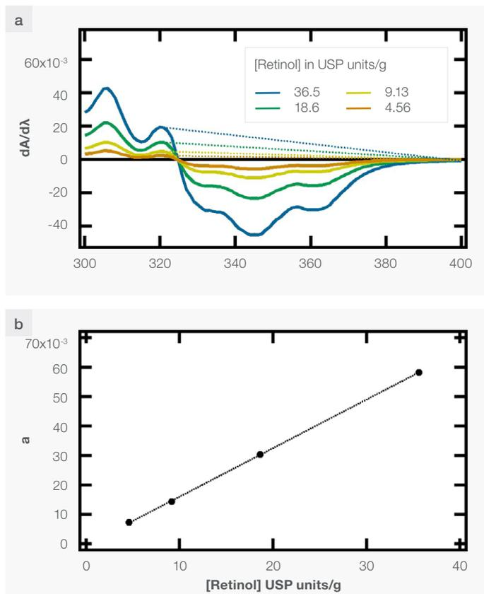
Figure 7. (a) First derivative spectra of all-trans-retinol of varying concentrations. Solid lines are the first derivative spectra and dashed lines are the tangent lines extrapolated using the relative maxima on either side of the minimum of interest. (b) Standard curve for “a” vs retinol concentration. All samples were measured using a 1.0 cm quartz cuvette.
