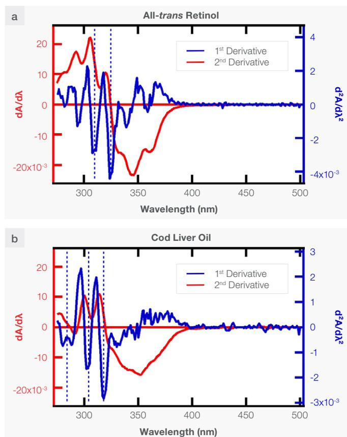
Figure 6. First and second derivative spectra of (a) all-*trans* retinol and (b) cod liver oil. The samples were measured using a 1.0 cm quartz cuvette.
