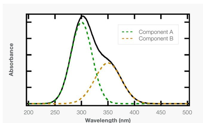
Figure 1. Calculated spectrum of a sample containing two species (black solid line), component A (green dashed line) and component B (orange dashed line).
