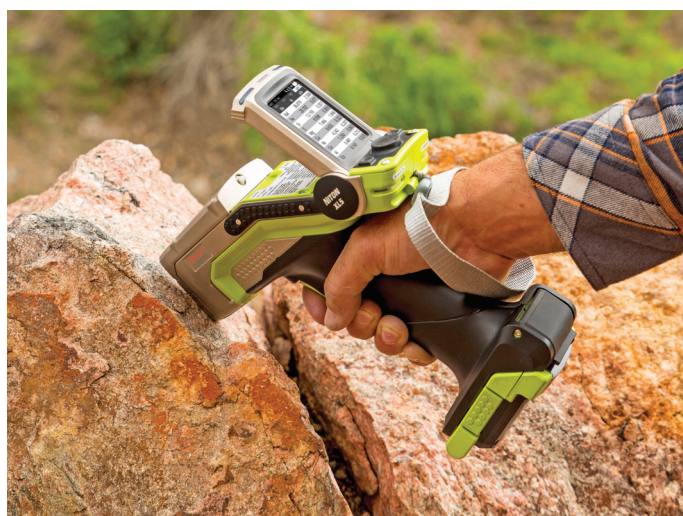
The Thermo Scientific Niton XL5 in use, analyzing a geological sample.
