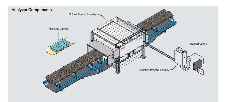
module contains control electronics for the neutron generator and incorporates all necessary safety features.
