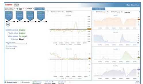
The main COBOS screen displays all the key inputs to and outputs from the system, along with trend lines on actual coal quality for each of the control parameters.
