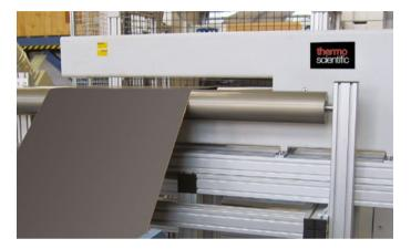
By measuring the distance to the sheet surface, the measurement is completely independent of sheet composition. The Laser TX optical thickness gauge does not need an alloy table, it is ideal for service centers and cut-to-length warehouses that hold a variety of metal grades in their inventory. Additionally, the use of laser based sensors completely eliminates the need for semiannual regulatory inspections. There is no longer a need for a radiation safety program or licensing.
