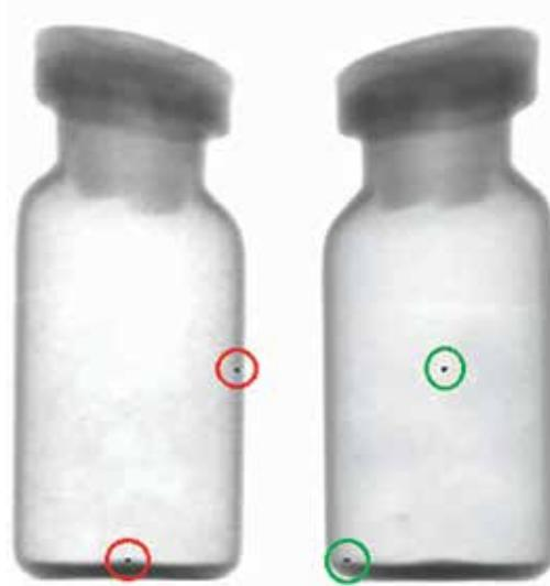
The POWERx D165 system inspects glass vials from two angles, finding contaminants in one view that are not visible in the other and increasing the probability of detection.
