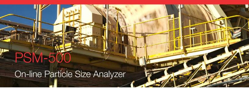
The Thermo Scientific Particle Size Analyzer PSM-500, provides real time, in-stream particle analysis of up to three streams. Measuring up to five particle size fractions simultaneously.
