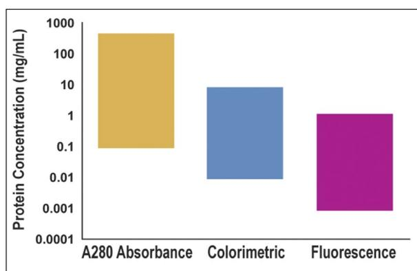
Figure 2: Comparison of the approximate dynamic ranges associated with the various protein quantification methods using a NanoDrop spectrophotometer or spectrofluorometer.
