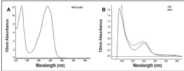
Figure 3: Influence of buffers on direct UV A280 protein measurements, A) Absorbance of 0.5× RIPA buffer (instrument blanked using water), B) Absorbance of the same protein sample in either 0.5× PBS or 0.5× RIPA buffer (blank and sample measurement performed using the same buffer). *Note that even when using appropriate blank, the absorbances of the two samples are not the same.*
