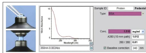
Figure 1: Left: loading of a 2  $\mu\text{L}$  protein sample on the measurement pedestal, Middle: liquid column between pedestals during sample measurement, Right: software output, showing both spectra and numerical data.
