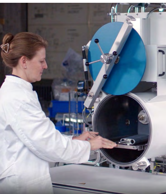
Figure 1: The HAAKE Viscotester iQ Rheometer can be conveniently transferred to the glovebox via an antechamber.
