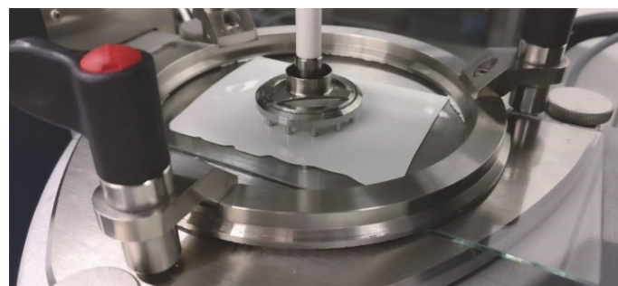
Figure 2. A glass plate with coating fixed into a Thermo Scientific™ HAAKE™ MARS™ Rheometer with the special holder. The rotor is in measuring position with the tips of the pins in the coating.
