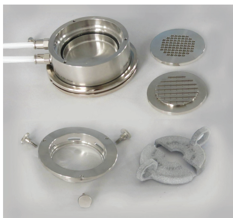
Figure 1. Components of the measuring cell (from left to right, top to bottom): measuring cell with hose connectors for a circulator, serrated measuring plate and perforated plate, mounting ring with 3 thumbscrews, two-parts sample hood.
