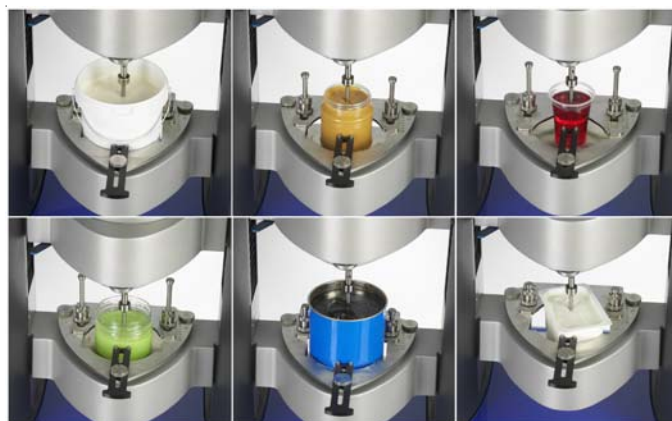
Figure 2: Universal container holder built in the HAAKE MARS Rheometer with selection of original containers.
