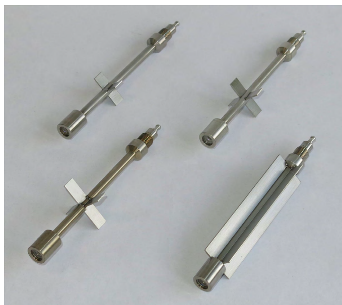
Figure 1: Vane rotors with a blade height of 8.8 mm with different diameters of 25 mm (upper left) and 30 mm (upper right), vane rotor with a blade height of 8.8 mm and a diameter of 36 mm (lower left), vane rotor with a blade height of 93 mm and a diameter of 25 mm (lower right).
