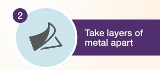
Disassemble scrap first and take layers of metal apart to accurately identify precious metals, varying alloy grades, and potentially hazardous metals such as lead.
