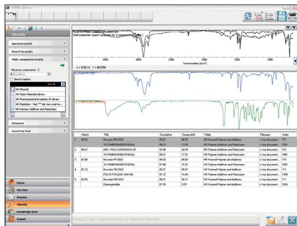
Figure 6: OMNIC Spectra multi-component identification of a polymer material fragment. The main compound is an acrylonitrile styrene butadiene techno-polymer (ABS) and several other peaks, which would not be identified by a simple search algorithm, match the spectrum of a bromide bis-phenol flame retardant.
