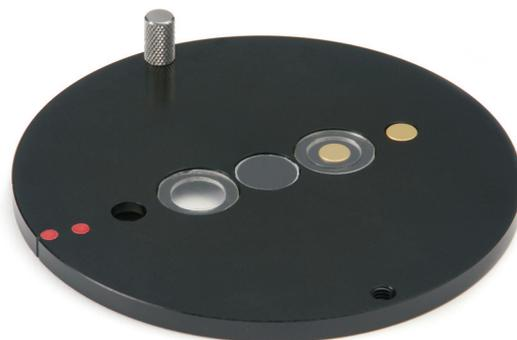
Figure 1: Performance verification plate for microscopes. The plate includes NIST traceable polystyrene standards and predefined locations for background collections offering a comprehensive performance verification test in any sampling mode, including transmission, reflection and micro-ATR. Performance verification is fully automated for consistency of experimental conditions.
