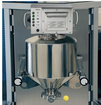
The Thermo Scientific Antaris Target blend analyzer provides blend end-point determination and confirmation of blend uniformity for tablet manufacturing.
