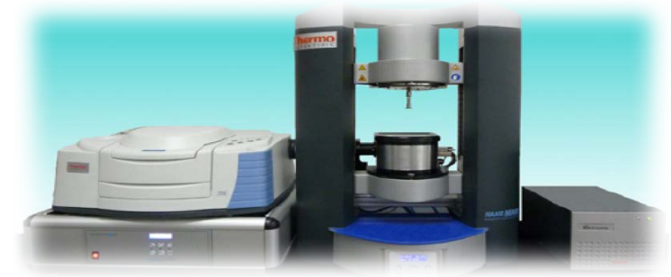
Rheonaut with Thermo Scientific™ Nicolet™ iS™ 10 FT-IR
