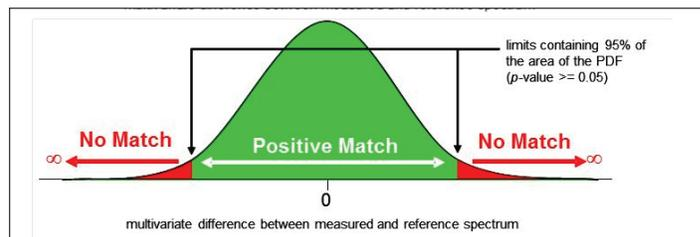
Figure 4. TruScan GP Positive Match/No Match univariate t-distribution.
