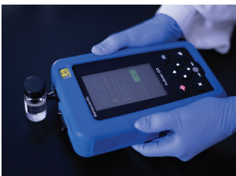
The Thermo Scientific TruScan™ G3 Handheld Raman Analyzer
