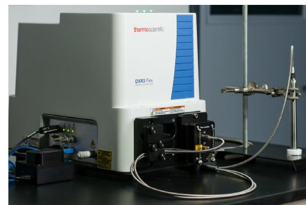
Figure 2f. The Thermo Scientific DXR3 Flex Raman Spectrometer.
