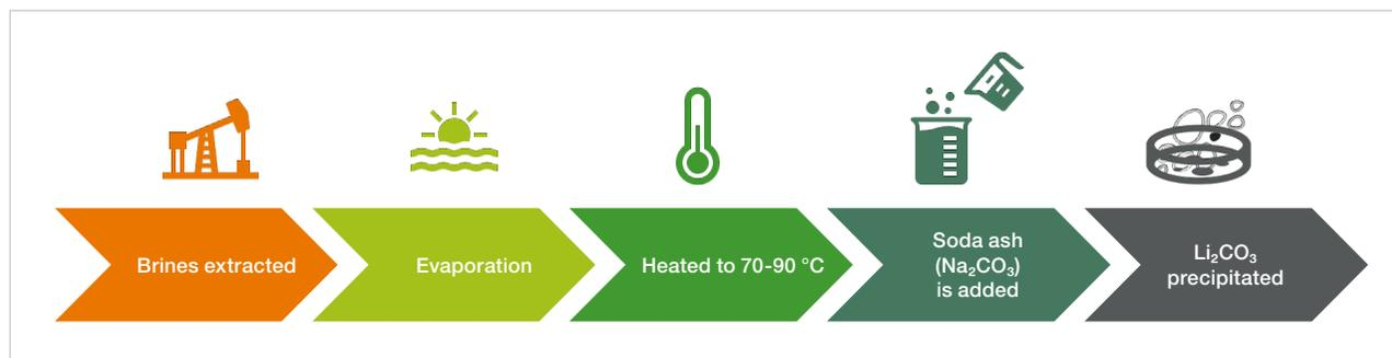
Figure 2b. Diagram of the process flow for lithium mining.
