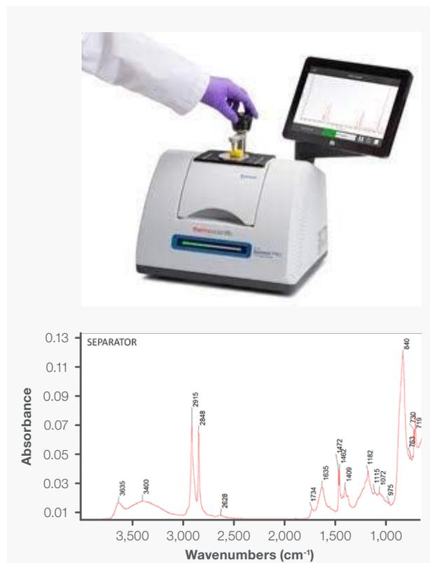
Figure 7d. Analysis of simple polymer by FTIR.
