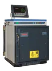
contamination before leaving a radiological controlled area. The SAM12 small article monitor readily measures down to clearance levels less than 80 Bq (5,000 DPM), but adds sophisticated new electronics allowing dynamic discrimination between natural and manmade radiations, as well as a unique feature for Co-60 monitoring. Measurement of fixed, smearable, internal and
