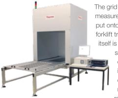
The grid boxes to be measured can simply be put onto the carriage by a forklift truck. The carriage itself is seated on bearings so that the grid boxes can easily be moved into and out of the cavity. Costly door mechanics and floor reinforcement usually
