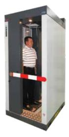
with an active area of 600 cm2. Four detectors exclusively monitor the hands. The foot detector has an active area of 570 cm2. The overhead detector comes with an auto retracting overhead pull-down head detector.
