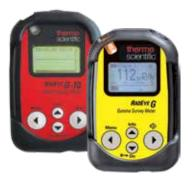
guarantees excellent linearity over 6 decades of radiation intensity: from background level to 1 Sv/h (10 R/h) - with overrange indication up to 1000 R/h. The RadEye G-10 version incorporates a different energy filter in order to achieve a Sievert response curve according to ambient equivalent dose rate H\*(10).
