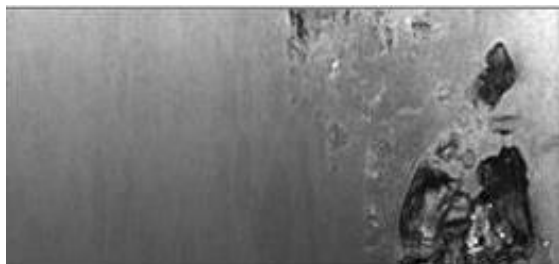
Figure 10. Photo of 40 mm void detected by SIPRO in hot strip mill running at 10 m/s
