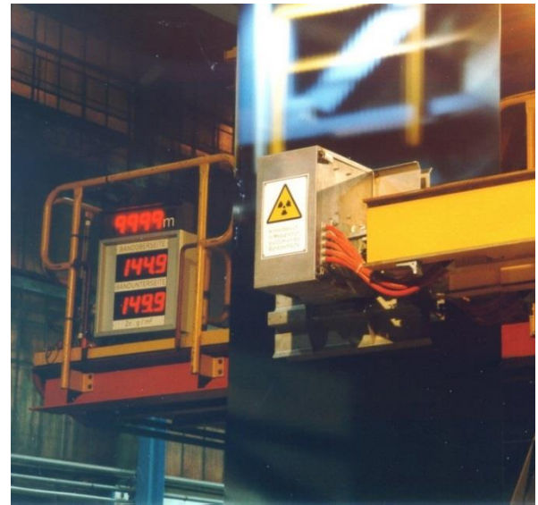
Figure 8. Immediate check of the adjustments of the coating device. The actual coating weight of top and bottom side are displayed
