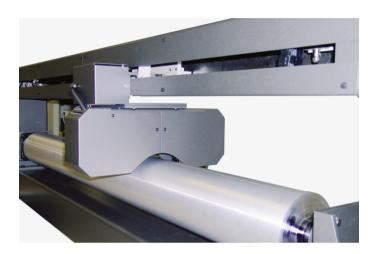
The ShadowMaster direct thickness sensor provides non-contact, online thickness measurement of a moving web. The sensor is designed to deliver accurate thickness measurement of materials up to 6500 microns (260 mils) and the measurement package comprises optical, inductive, and temperature sensors.
