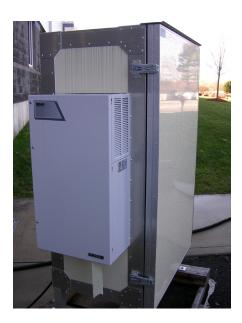
The Complete Outdoor Enclosure for the TEOM Series 1405 is a cost-effective alternative to permanent shelters especially in locations where a fixed shelter is not available for installation.
