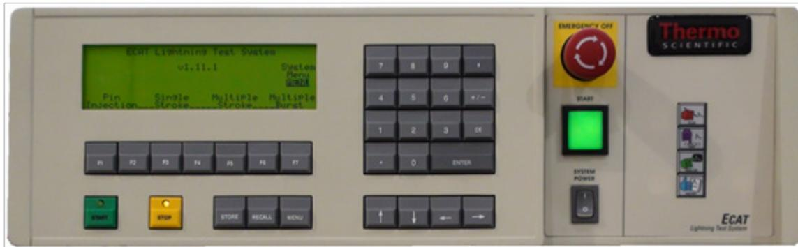
1. Select Test Type: Pin Injection, Single Stroke, Multiple Stroke or Multiple Burst
