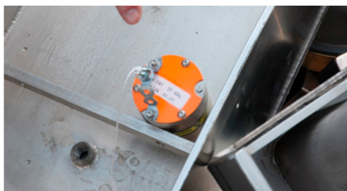
1 Ci Am-241 source in Tungsten shielding container
