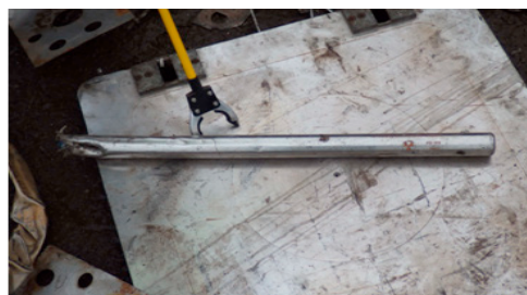
50 mCi AmBe industrial source found in steel scrap
