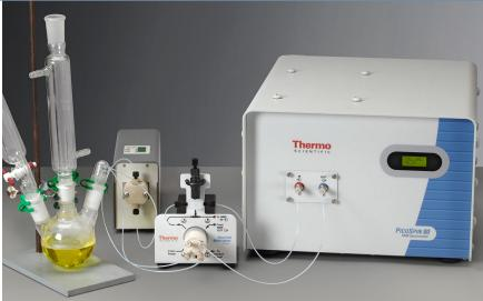
Adding a reaction monitoring accessory to the picoSpin 45 or the picoSpin 80 NMR spectrometer gives your students valuable hands-on experience of chemical reaction mechanisms, kinetics, thermodynamics, and other physical organic properties to complement the core of your undergraduate chemistry curriculum.
