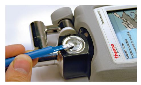
Thermo Scientific™ TruDefender™ analyzers are rugged, handheld FTIR systems for rapid identification of unknown chemicals including explosives, narcotics, toxic industrial chemicals and precursors. They bring the power of FTIR directly into the hazard zone, enabling the responder to analyze—and act—faster than ever before.
