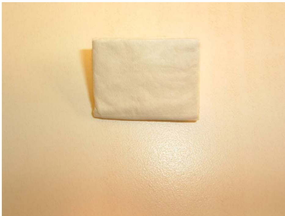
Figure 13: Wipe after fifth fold; the wipe should measure 1 x 1.5 inches
