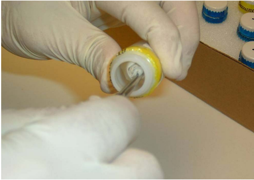
Figure 3: Carefully remove ELPAT wipe from sample tube
