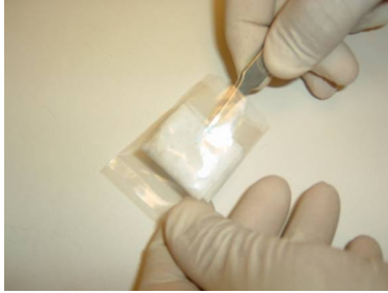
Figure 16: Use clean tweezers to transfer wipe
