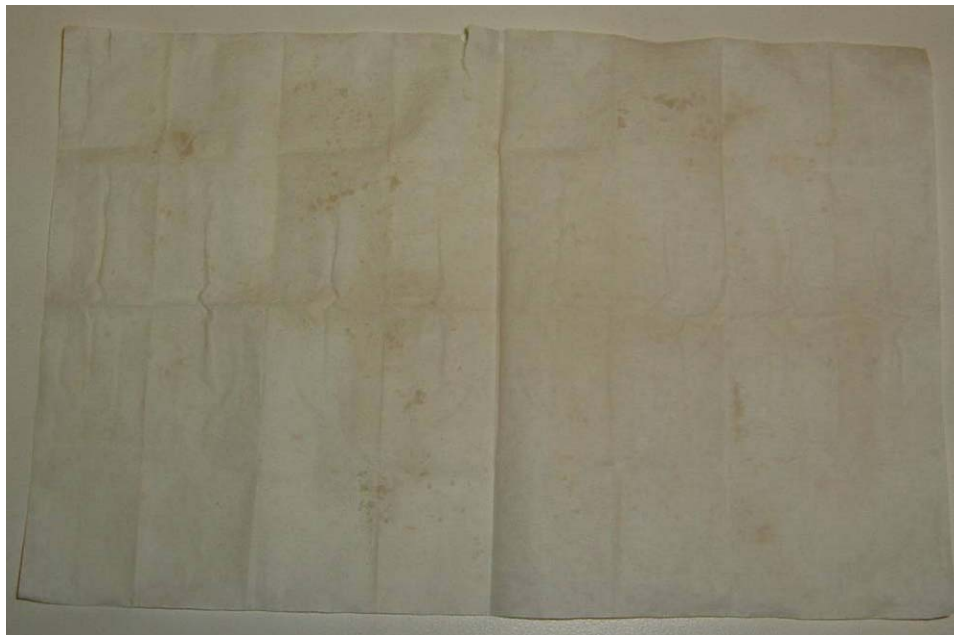
Figure 8: Evenly distributed lead on wipe, ready to fold
