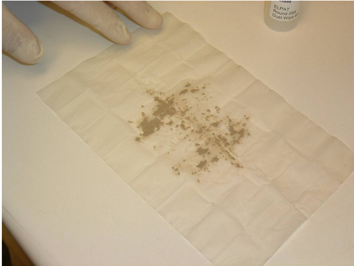
Figure 1: Uneven distribution of lead sample on ELPAT wipe
