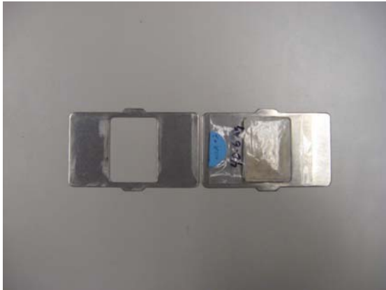
Figure 18a: Dust wipe in metal frame
