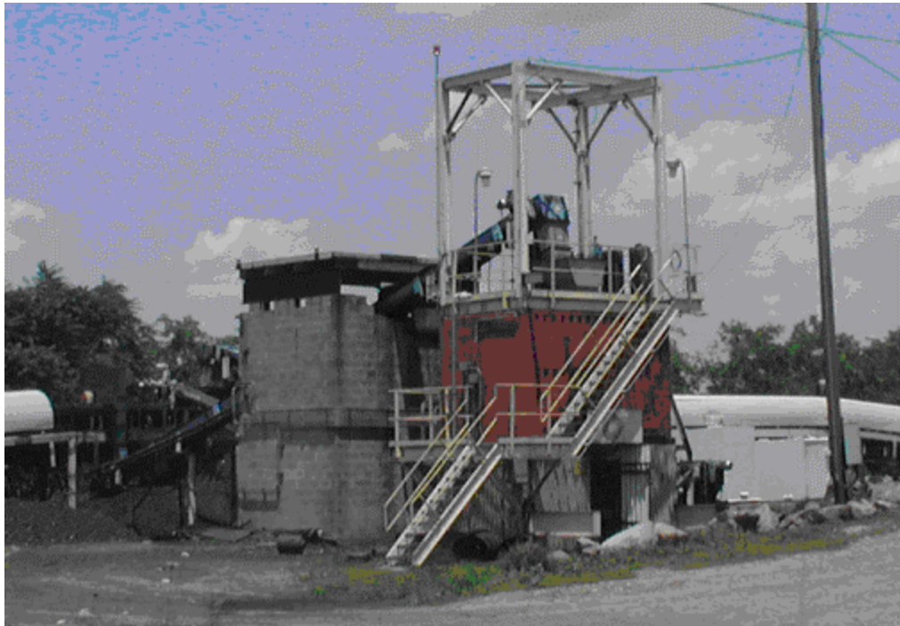
Figure 5. Gamma-Metrics 1812C Coal Analyzer near the overland belt.
