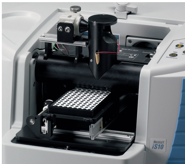
Figure 6: Micro-plate reader shown installed in the Nicolet iS10. Operation of the accessory is the same in either the Nicolet iS10 or Nicolet iZ10.
