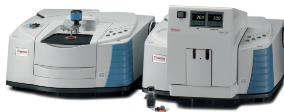
Figure 1: Nicolet iS10 with Smart iTR™ diamond ATR coupled with the Nicolet iZ10 and the TGA sampling accessory
